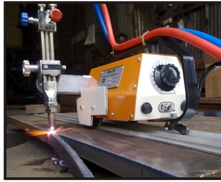
Maximum Cutting thickness upto 70mm
