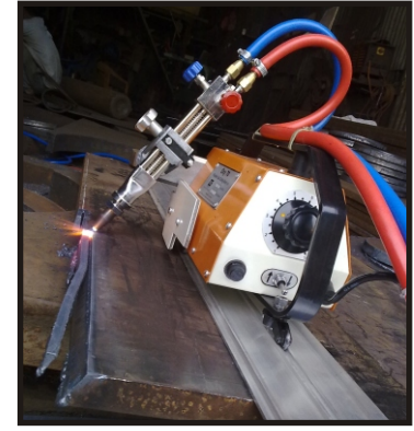
Bevel Cutting upto 45 Degree
